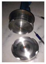
Implosive piston with rings, hydraulic dampener and cylinder head - designed for plasma injector.
