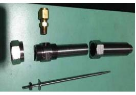
Injector expanded view without insulator or connected fuel and plasmoid inlet
