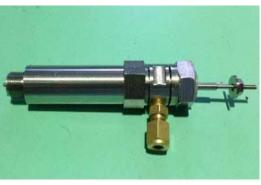
Injector without insulator with fuel and plasmoid inlet
