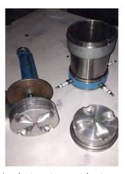
Implosive piston with rings, hydraulic dampener and cylinder head. Cylinder with 4 platinum fusion sparkplugs.
