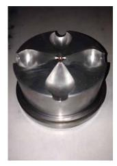
Implosive cylinder head concentrating force into a central tungsten carbide sphere.
